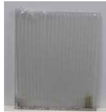
Figure 2: Aged multi wall PC sheet.
