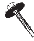
#12-14 x 1-1/4" HWH w/1-1/8" Oversize Bonded Washer (pre-drilling w/oversize holes required on all sheets)
