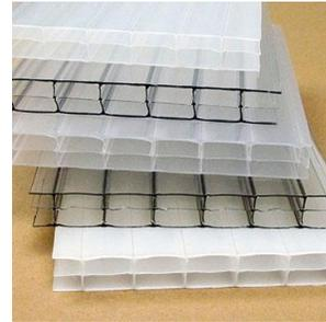
LEXAN™ THERMOCLEAR™ 16mm has three walls and two "air-trapping" layers, increasing its thermal insulation properties and its ability to withstand higher wind and snow loads.
