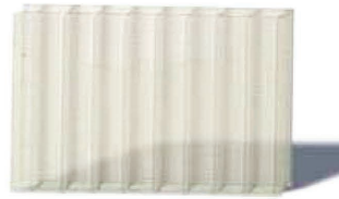
Sample 2 - Delta YI=5 LEXAN™ THERMOCLEAR™ 15
