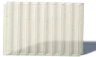
Sample 2 - Delta YI=5 LEXAN™ THERMOCLEAR™ 15
